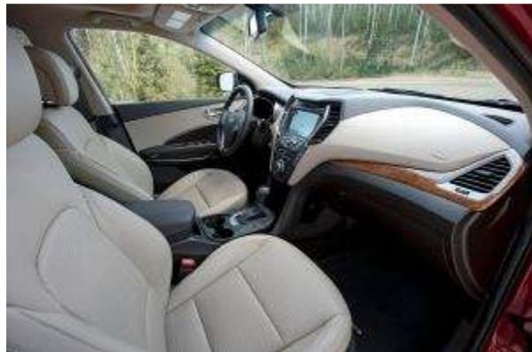
The center section has the CD player, satellite radio, climate and Bluetooth connections. The test car had a four-inch screen which served the backup camera. There was
